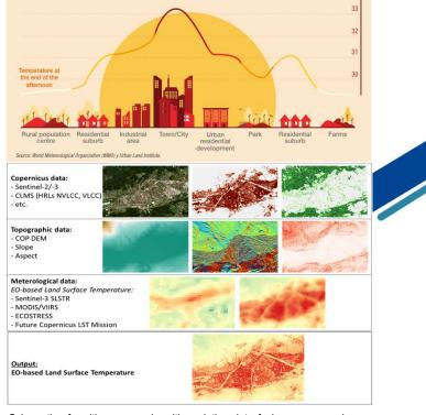
Schematic of multi-sensor and multi-resolution data fusion process using an ML-based regression modelling approach. The schematic shows that a combination of HRL NVLCC IMD and HRL VLCC TCD, topographic, and EO-based datasets is used to train an Al-based machine learning model to downscale the Land Surface Temperature (LST).
