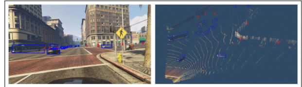
Figure 1: Annotated image and point cloud pair in PreSIL generated dataset. Reproduced from: [7].
