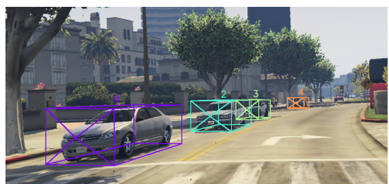
Figure 2: Visualization of object tracking in the PreSIL-generated dataset using PC3T.
