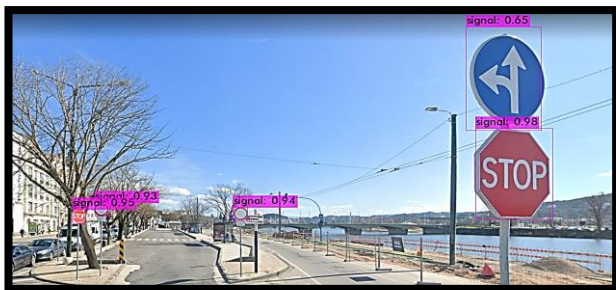
Figure 2: Results of the application of the traffic sign detection algorithm. (image from Coimbra).
