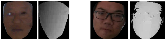
Figure 1: Comparison between RGB and depth images of a print attack (left) and a bonafide face (right). Note that the depth images aren't of great quality, not being able to capture the eyes cut out of the print attack and not giving much detail to the bonafide case, but being possible to notice the differences. Images selected from the CASIA-SURF dataset [10].
