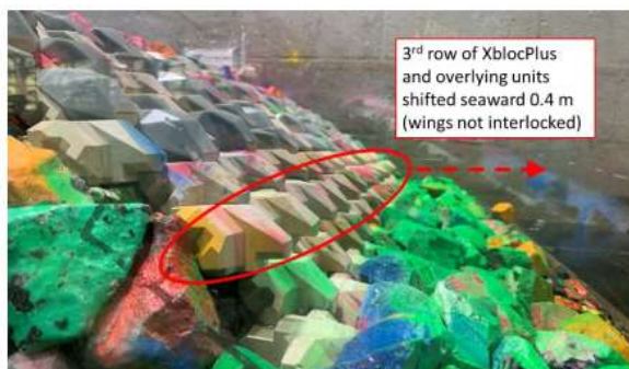
Figure 3 Post seismic event profile constructed in the laboratory with the secondary armour and 3rd row of XblocPlus displaced forward with their noses and wings not interlocked.
