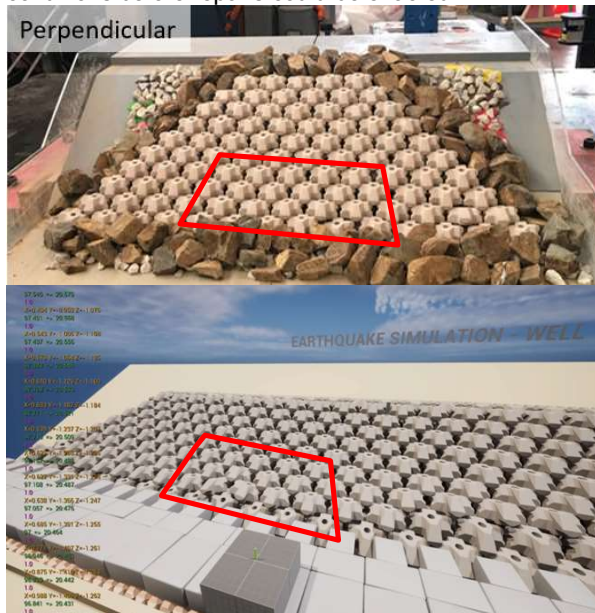
Figure 2 Example of the XblocPlus Revetment following a design seismic event using a shake table (1D - upper) and Unreal Engine (3D - lower).
