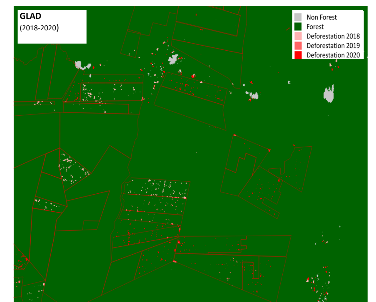
Forest change detection by the GLAD system of Global Forest Watch in the same time period. The system detects deforestation, but hardly any forest degradation.
