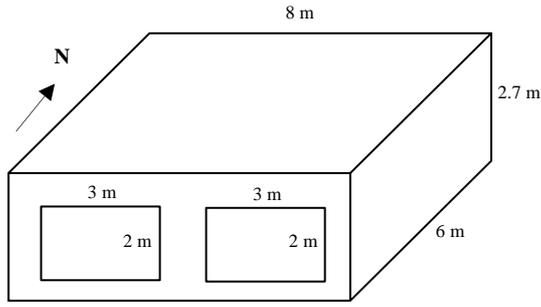
Figure 1: Building geometry of test cases based on the ANSI/ASHRAE Standard 140.
