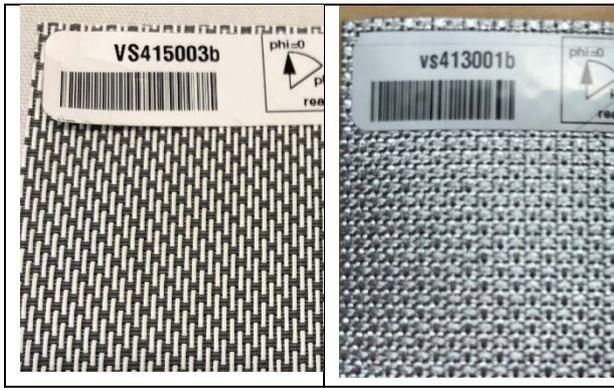
Figure 4: Outdoor-facing surfaces of measured samples from fabric A (left) and fabric B (right). The labels with dimensions of 38 mm x 13 mm give an indication of scale.
