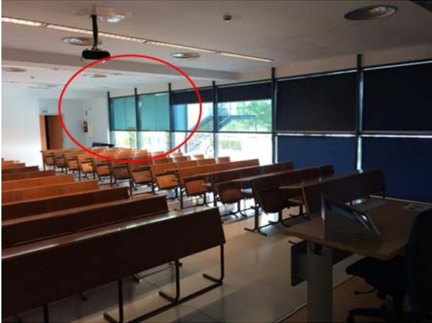
Figure 1: Informal retrofit action in a classroom to prevent glare. A formal retrofit action, consisting of a reflective film applied to the exterior glass pane, had already been undertaken for the upper partition.
