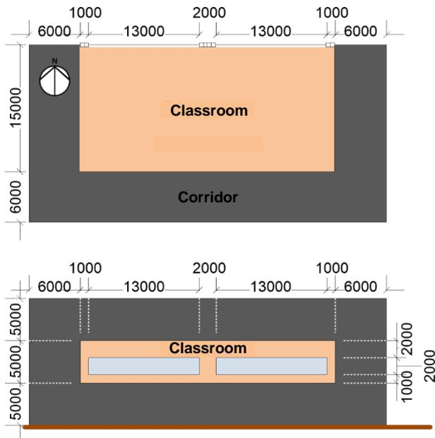
Figure 1: Floor plan and elevation views of the modelled classroom building; units in mm
