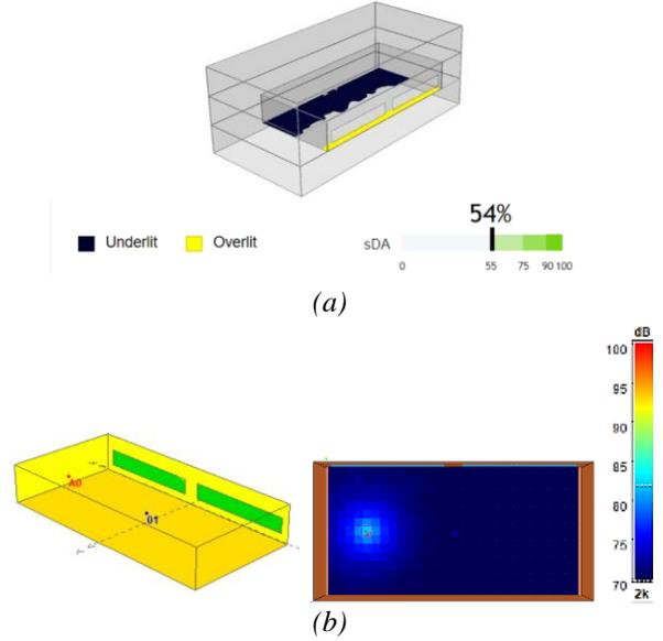
Figure 2: Typical visualisations of (a) the daylighting simulation results in *Sefaira* and (b) the acoustic simulation results in *CATT v9*
