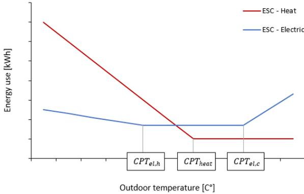
Figure 1: Energy signature curve concept for heating and electric demand various building categories.
