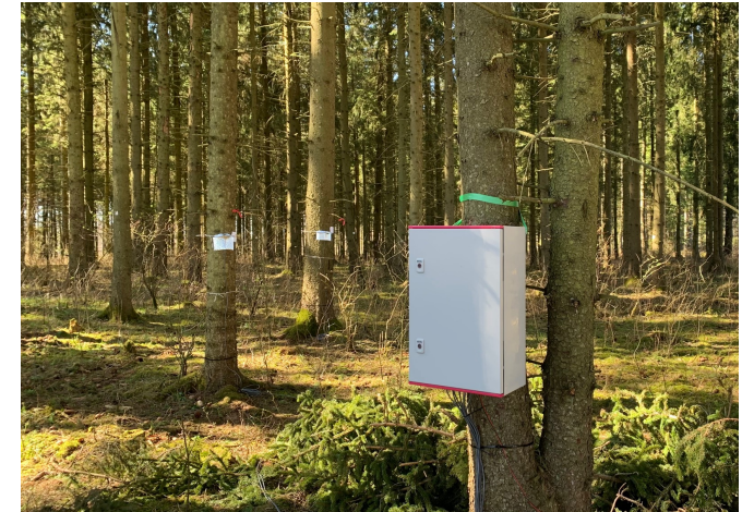
Stations monitoring sap flow changes during bark beetle attacks
