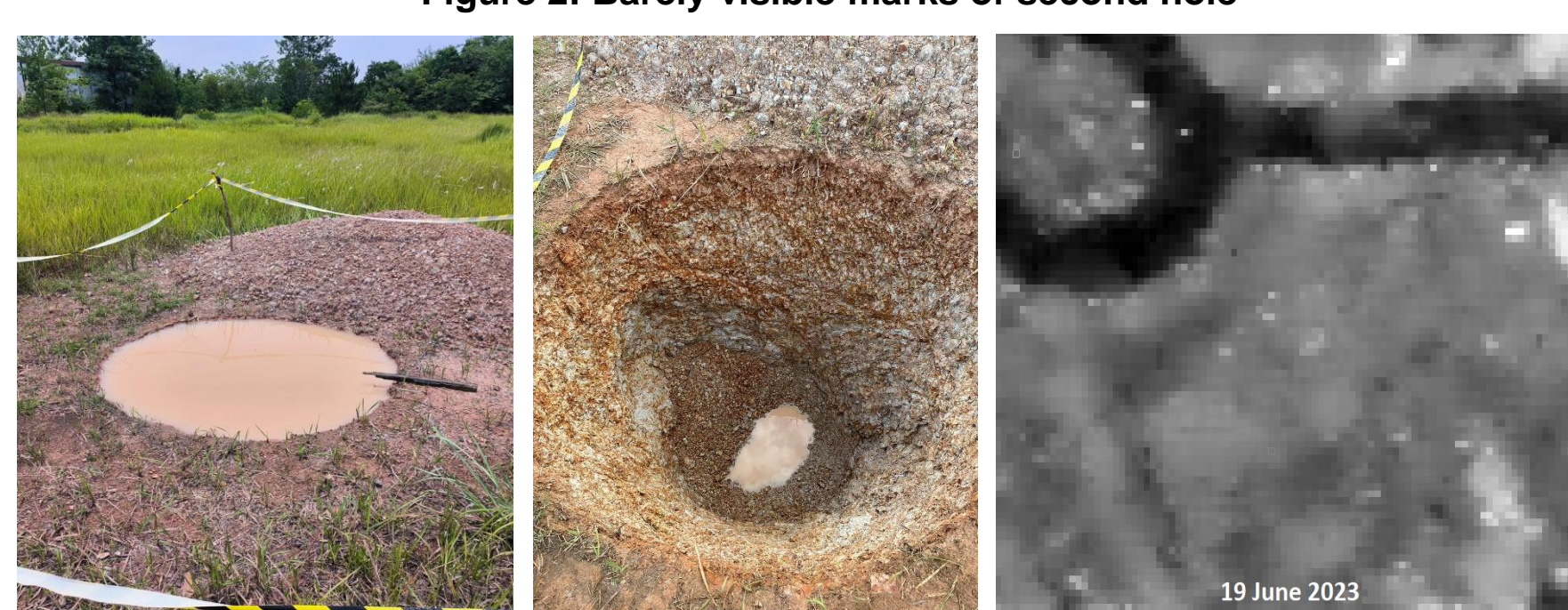
Figure 3: Image taken after the rainfall. Soil slide after rain changed the measures of the hole.
