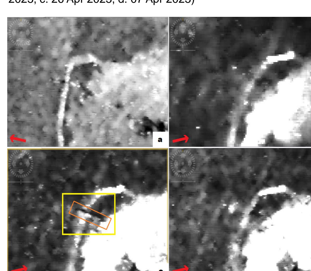
Figure 17: Filtered SAR images of the collapsed column. Orange polygon shows the column on the ground. (SAR Acquisition dates: a: 12 Mar 2023, b: 21 Apr 2023, c: 26 Apr 2023, d: 07 Apr 2023)
